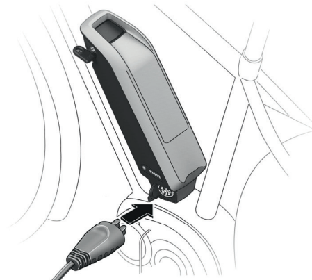
Image 28: Plugging charger plug in charge socket on the bottom part of the battery holder
