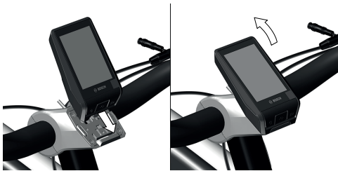
Image 14A: Inserting the display
